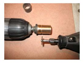
You then use a fine sanding drum on the Dremel (a dowel & emery paper would work) to take a little off the inside of the bushing so that it will fit properly on the bike. You don't need to take much off, probably only a few thousandths of an inch. I don't think you need a picture of this.
