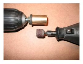
Turning the outer diameter to size. Both the drill and the Dremel tool are turned on to do this.
