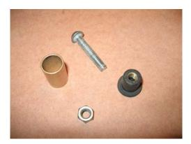
The piece on the left is a 3/4 inch od, 5/8 inch id bronze bushing. You can get these at most big hardware stores; they cost a couple of bucks. The other piece is a well nut. It should be sized to fit the bushing as in the next pic. The screw goes in the well nut, and the nut holds the screw in place.
