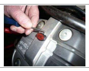
Pic 2: Undo the 3mm hex bolt that holds on the HT lead cover and remove it.
