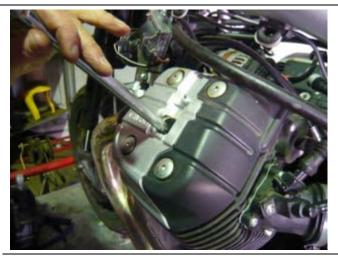
Pic 4A - 4B: Using an extension and plug socket, extract the plug.
