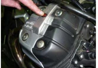
*Pic 24:* Re-install the bung on the front of the belt cover.
