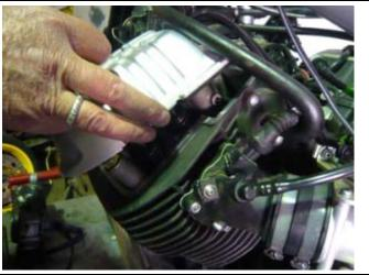
*Pic 9:* Pry out the rubber bung from the front of the alternator belt cover.
