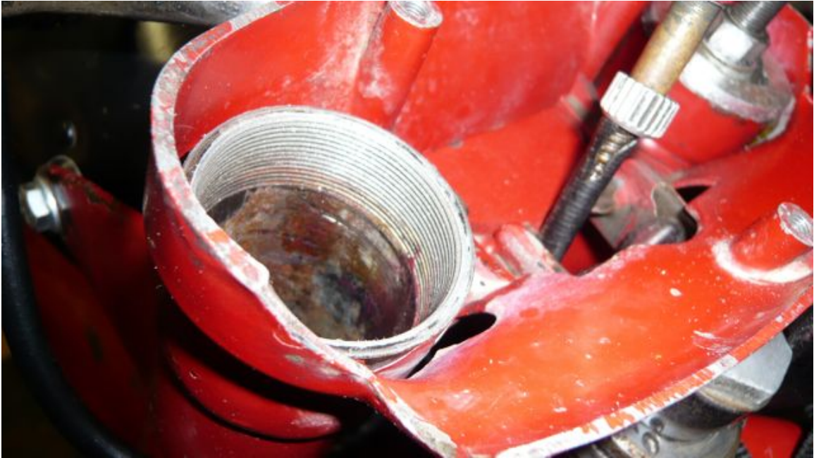
Top of the fork leg, showing some corrosion.
