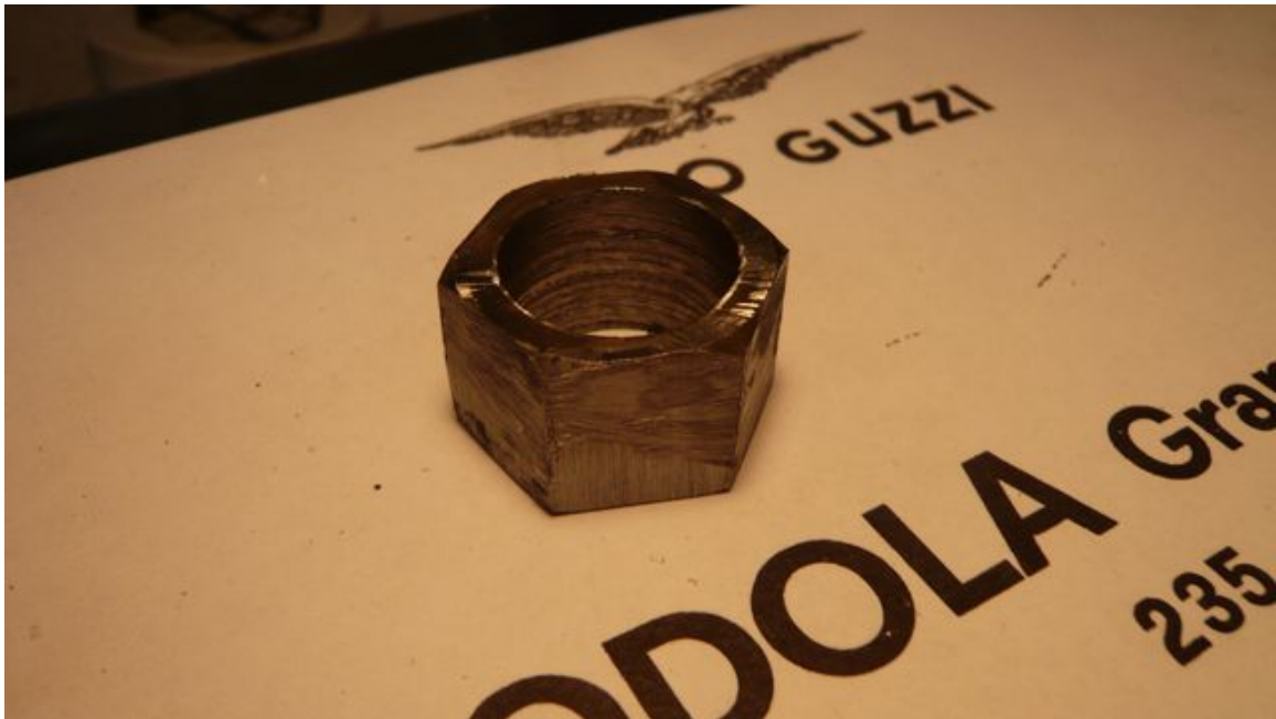
The “Special tool” 29mm flat to flat with a 20mm hole. Machined from a 3/4” heavy nut.
