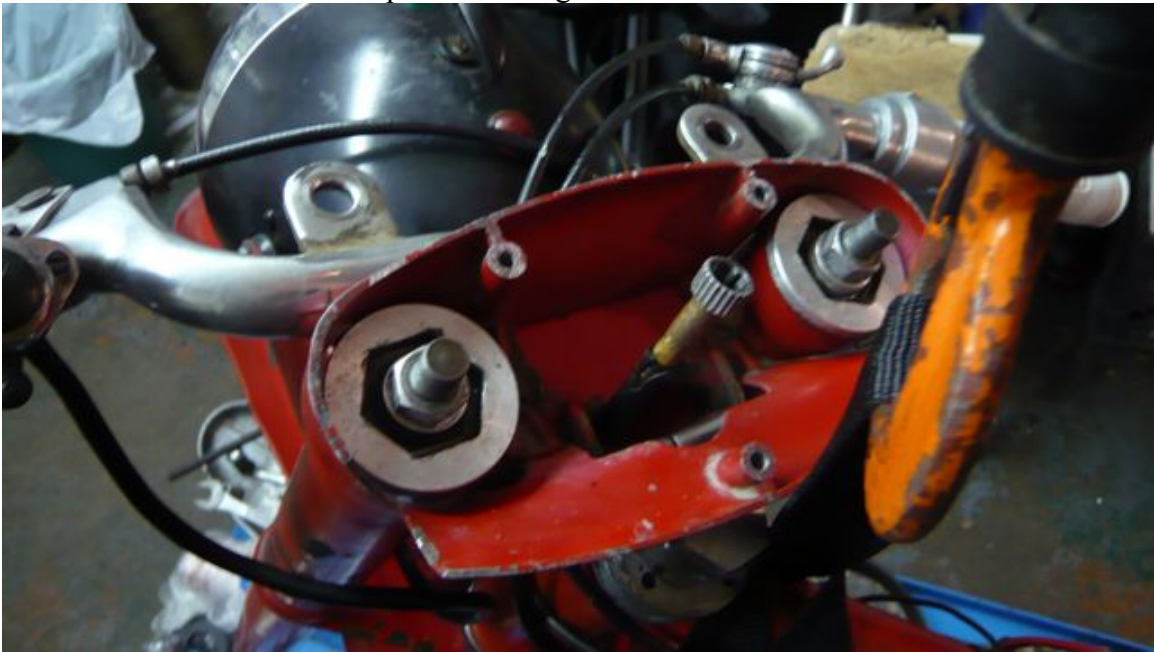
Handlebars are removed exposing the 29mm internal hex caps
