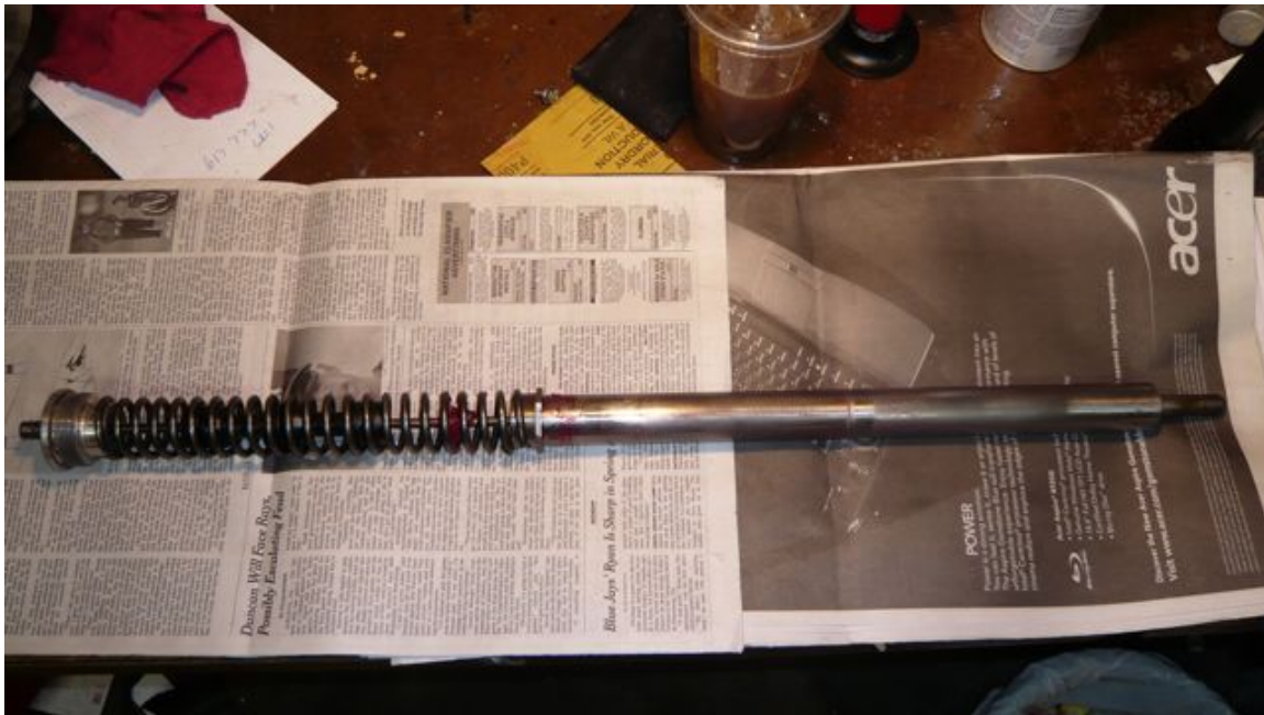
Fork tube complete, including tube, spring, damper, damper rod and cap
