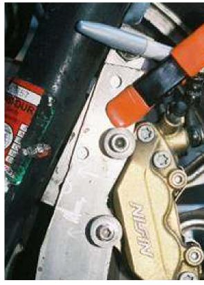
After drilling the holes, transfer the location to the second piece, mark, center punch, and drill. I chose 5/16<sup>th</sup> holes and used 8.8 hardened bolts and nuts plus Loctite.
