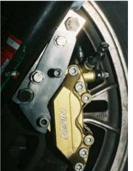
Press the brake pad surface against the other side of the rotor and identify where on the edge it hits. Half the distance between where the caliper hits while pressed against the rotor from each side is the thickness needed to shim the caliper to center it on the rotor. In this case, the caliper needs to be moved out from the wheel. Depending on the caliper used, it may be necessary to move the caliper in towards the wheel.
