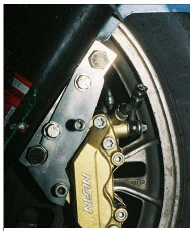
This is the second mount build, solely for the purpose of these photos. If I connected this caliper to the linked brake system, the proportioning would be far to much to the front wheel when engaging the foot brake. I'm more likely to try and mount this caliper on the rear rotor.
