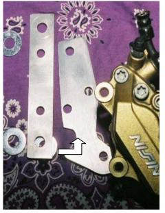
The finished mount pieces with all the excess metal removed, sharp edges rounded and all burrs filed flat. Note the arrow: I trimmed this so the mount bolt through piece A would not be half on piece B. Had I trimmed piece B correctly, the bolt would have passed fully through both pieces as it does on the first mount (see the photo of the right side caliper for detail).
