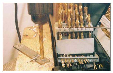
15/64th is as close as I could come to the stock bolt that originally held the caliper to the fork lower tube on my '79 SP1000. After drilling second hole in piece A, mount it to the lower fork tube "ears" to check fit. If the bolts bind, file the hole as necessary.
