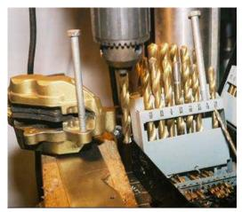
Size the holes carefully. For this caliper, 5/16<sup>th</sup> is about as close as I can come to the metric size. As before, I center punched the location, then transferred the distance between centers with a compass. drilled a pilot hole with a small bit before drilling with the full size drill.
