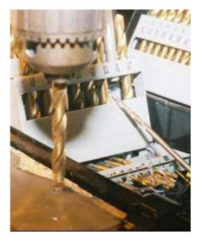
Drill a pilot hole, then the full size hole for only one end of the caliper.
