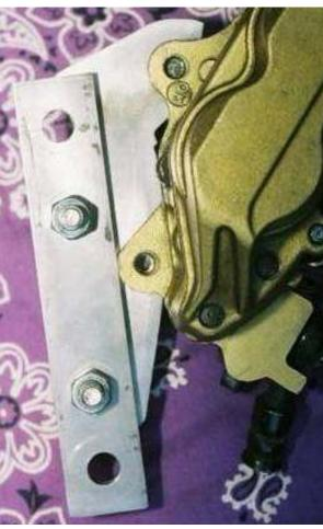
Check the fit and file if necessary to allow both bolts to enter without binding. For now, ignore that the two pieces A & B have been drilled and bolted together as this will come later.
