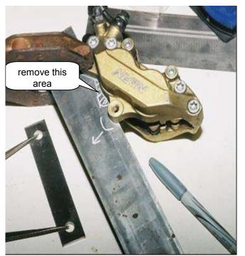
Layout mount position for caliper to piece B. This caliper requires some material be removed for the mounting holes to be fully on the metal. You can use a grinder, metal cutting jig saw or abrasive saw to remove the material. Remove small amounts and periodically check what remains to be removed.
