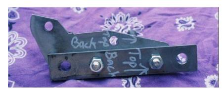
The fitted mounting plates together. Be sure to mark the pieces so they won't inadvertently be assembled incorrectly changing the alignment of the caliper to the rotor.
