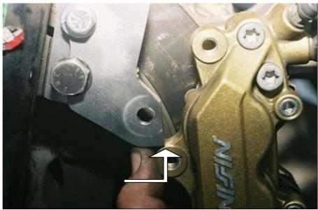
Bolt piece A and B together and then to the fork lower. With the brake pads pressed in as far as they will go or removed, press the brake pad surface of the caliper against one side of the rotor and identify where on the edge of the mount it hits.
